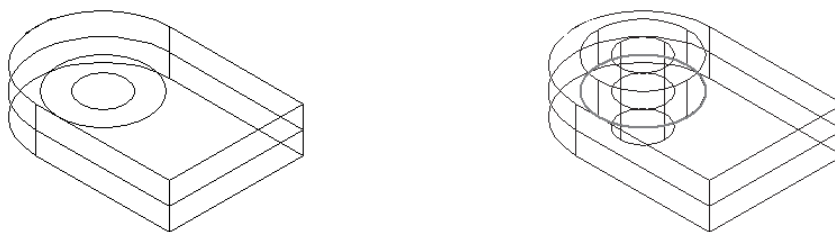
Left: TurboCAD's two-sided extrusion
